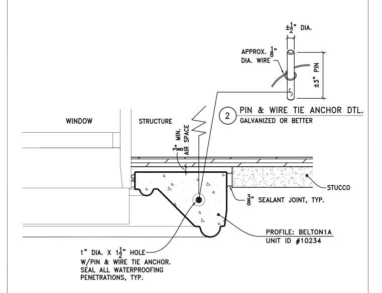
CAST STONE JAMB ATTACHMENT AT STUCCO WITH PIN & WIRE TIE ANCHOR
